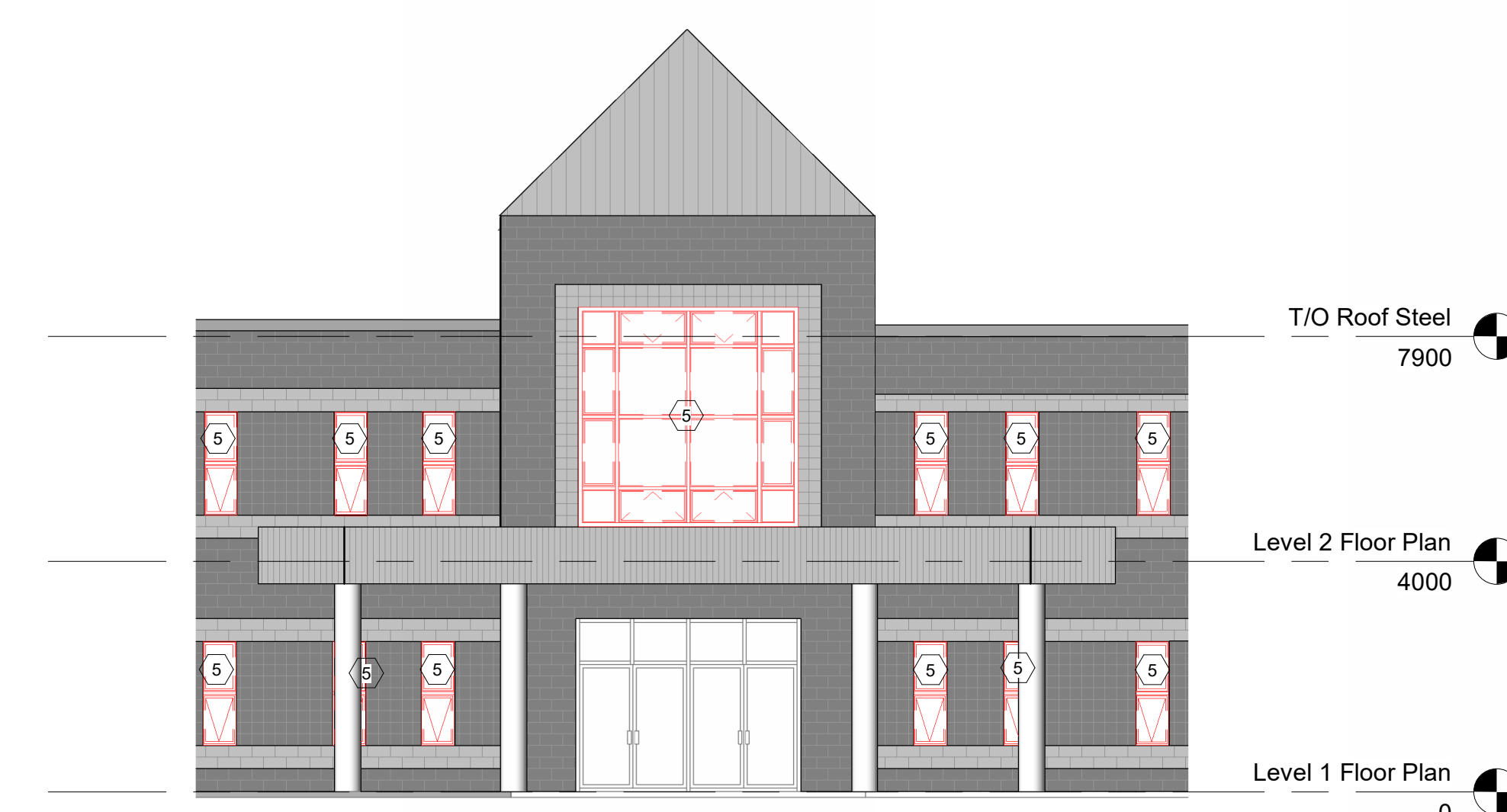
7 Partial Elevation - Main Entrance - Demolition 1 : 100
