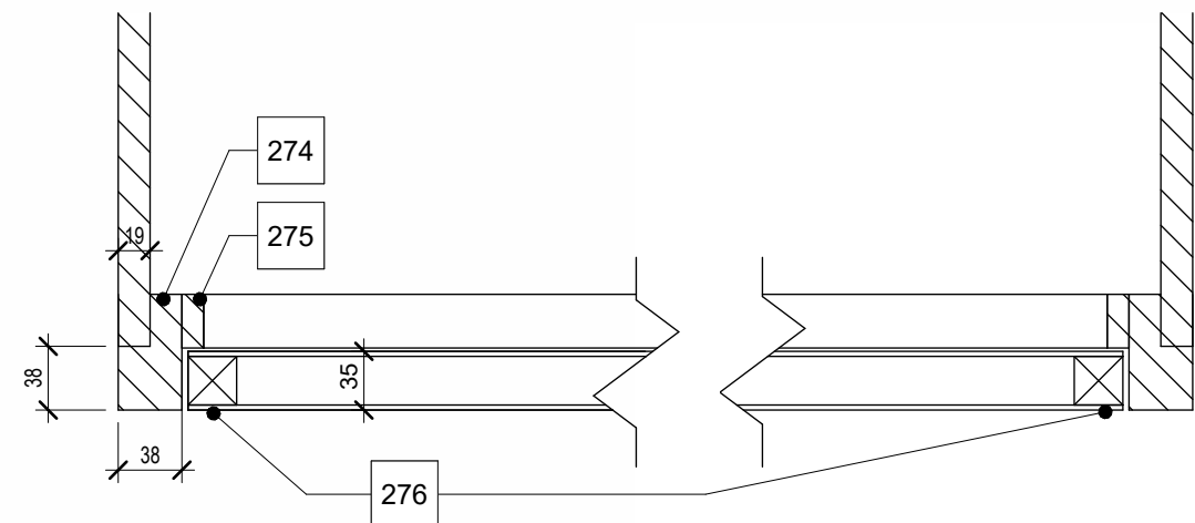
Classroom Storage Solid Frame - Plan Detail
