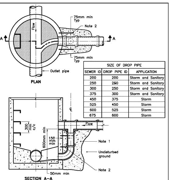
1 Concrete shall be placed to undisturbed ground and the outside face of the maintenance hole, but there shall be a minimum of 150mm of 15MPa concrete around the drop pipe. 2 Concrete shall be secured to the maintenance hole with 450mm long, 13mm diameter threaded rods and drilled expansion anchors down either
