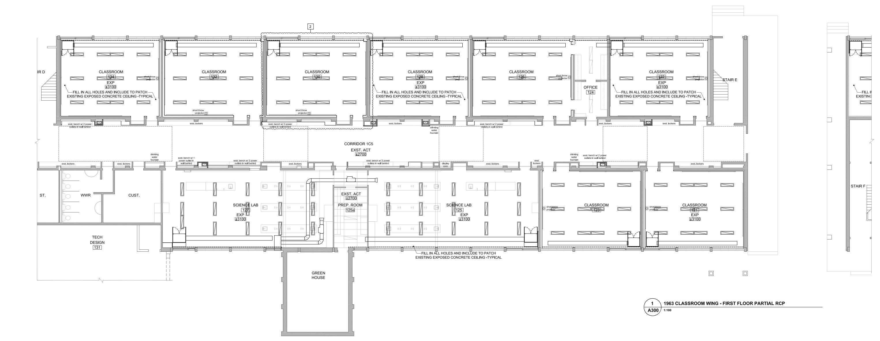
SHADED AREA INDICATES REMOVED LIGHT FIXTURE LOCATIONS. SC01 TO MAKE GOOD CONCRETE CEILING. TYPICAL IN ALL ROOMS.
