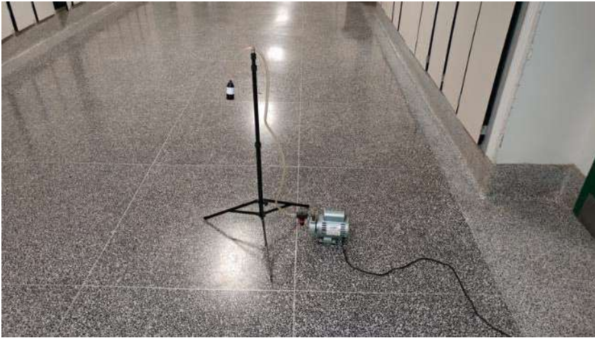
Photo 1: Air monitoring equipment Corridor adjacent Room 515.
