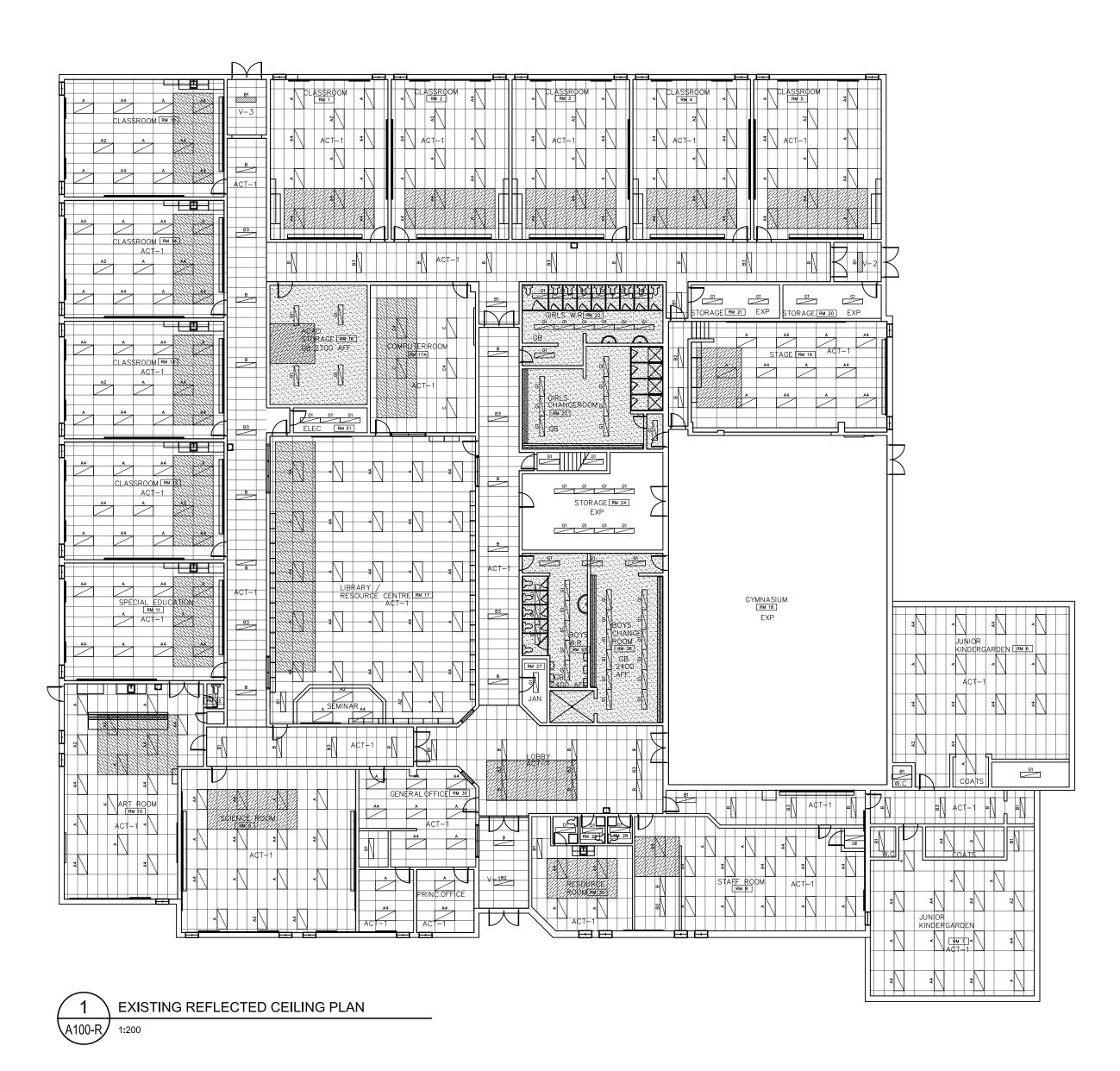
SHADED AREA TO HAVE MECHANICAL HEAT PUMPS INSTALLED, PORTION OF THE CEILING TO BE REMOVED CAREFULLY FOR INSTALLATION OF NEW HEAT PUMPS AND CEILING TO BE REINSTALLED AFTER (SCOPE TO BE INCLUDED IN SC01)
