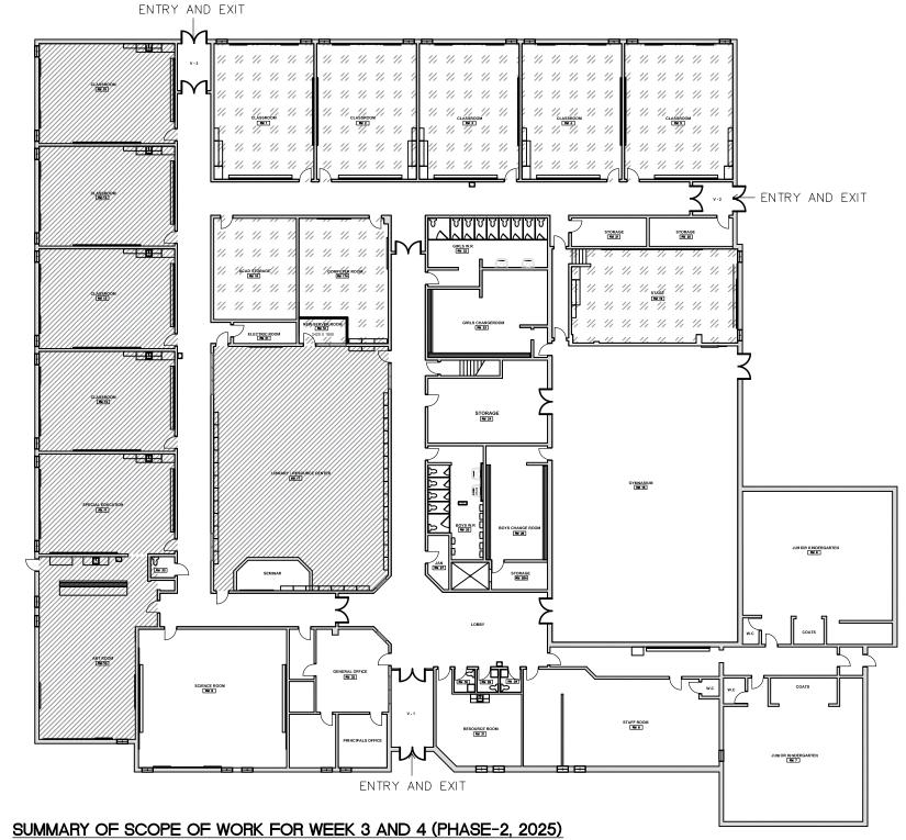
REMOVE AND DISCARD EXISTING CEILINGS, REPLACE ALL DUCTS AND ADD DIFFUSERS FOR EACH HEAT PUMP (SEE MECHANICAL AND ELECTRICAL). INSTALL NEW CEILING, INSTALL NEW LIGHTS ETC.
