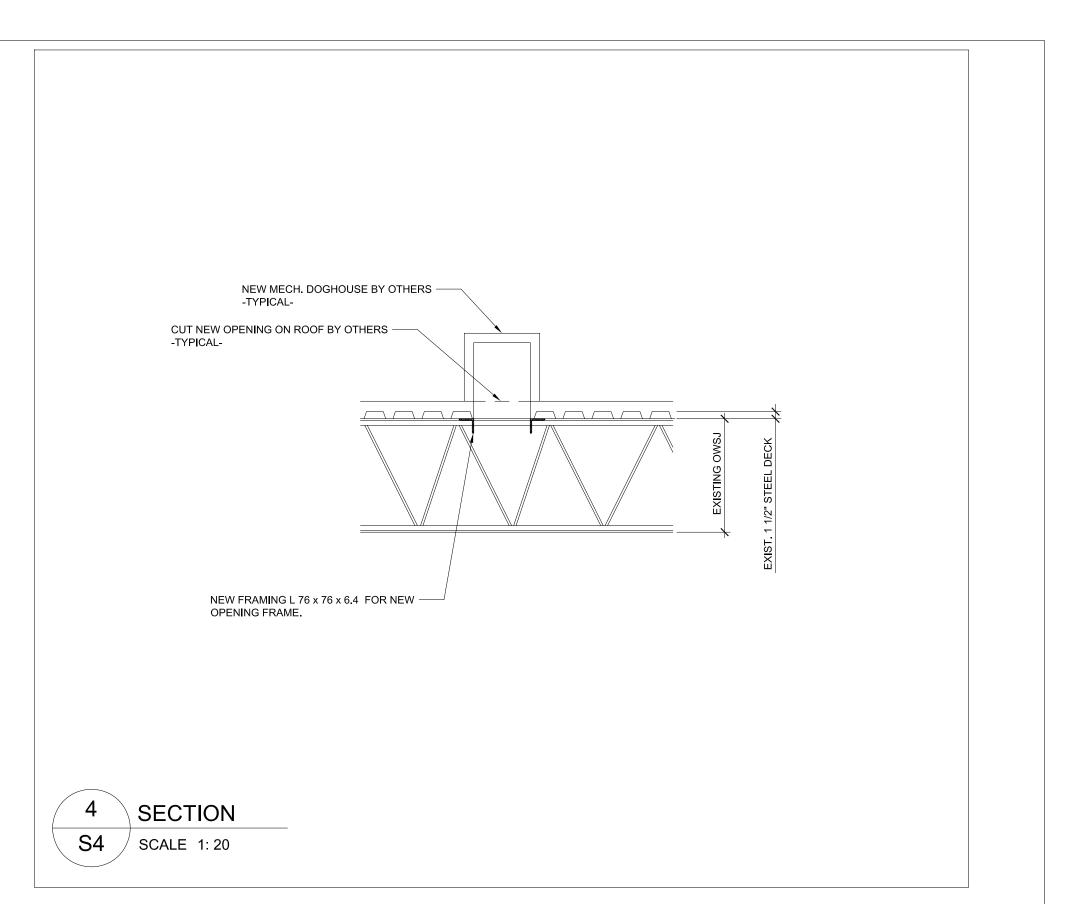
TYPICAL FRAMING FOR NEW ROOF OPENINGS ON EXISTING STEEL DECK ROOF.
