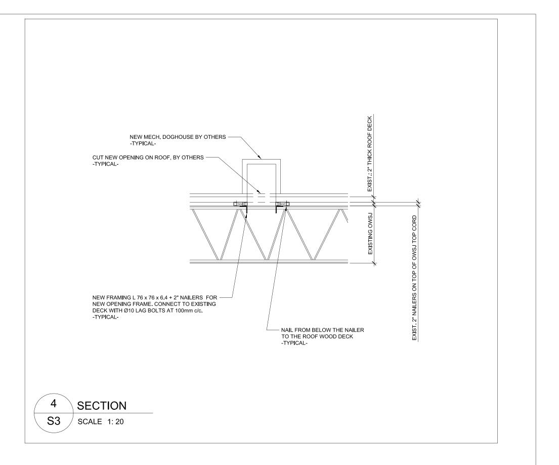
TYPICAL FRAMING FOR NEW ROOF OPENINGS ON EXISTING WOOD DECK ROOF.
