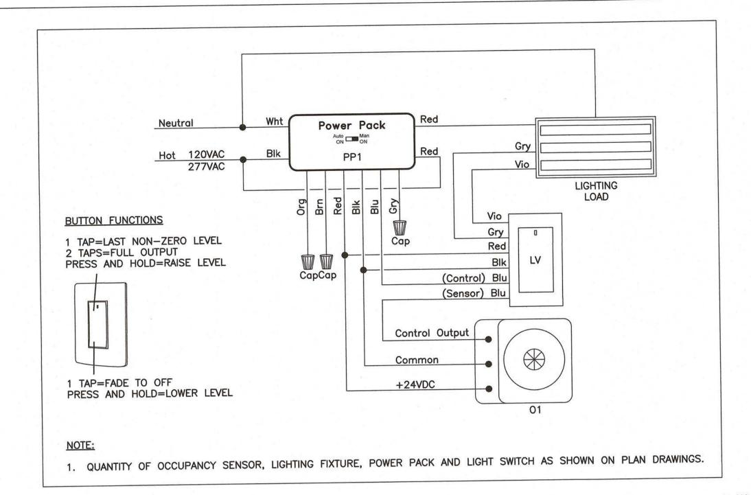
TYPICAL WIRING DIAGRAM FOR LOW VOLTAGE ON/OFF SWITCHING WITH 0-10V DIMMING
